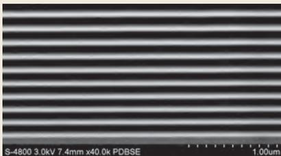
SEM image of an AlN layer with strong c-axis orientation
