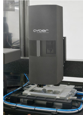
Sensor unit on top of heating stage with glass cover to protect sensor from heat
