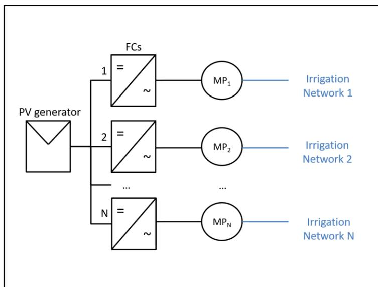
Figure 1 - Stand-alone PV systems: the irrigation system is fed by energy produced by PV generators. Figures depicted in black represent the electrical part, in blue the hydraulic part. FCs stands for frequency converters, while MP is for motor-pump.
