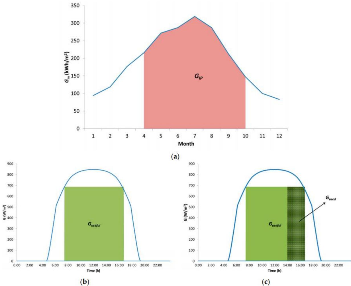
Figure 5. Graphical representation of the different irradiances considered: (a)  $\int G_{IP}$  is the irradiation during the irrigation period, (b)  $\int G_{useful}$  is the useful irradiation during the IP determined by the design of the PV irrigation system; and (c)  $\int G_{used}$  is the irradiation effectively used by the system.
