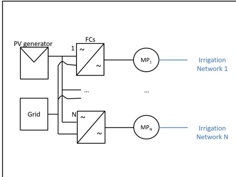
Figure 3 - Electric hybrid systems: hybridization among PV generators and the other sources is carried out in the electric part of the system.
