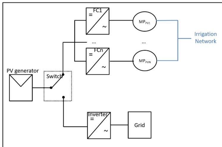
Figure 4 - Mixed systems: the system is a PV irrigation system during the irrigation period, and a grid-connected system outside the irrigation period. The switch allows the change between the two operating modes and, in the case of this figure, the switch is in the PV irrigation system position.
