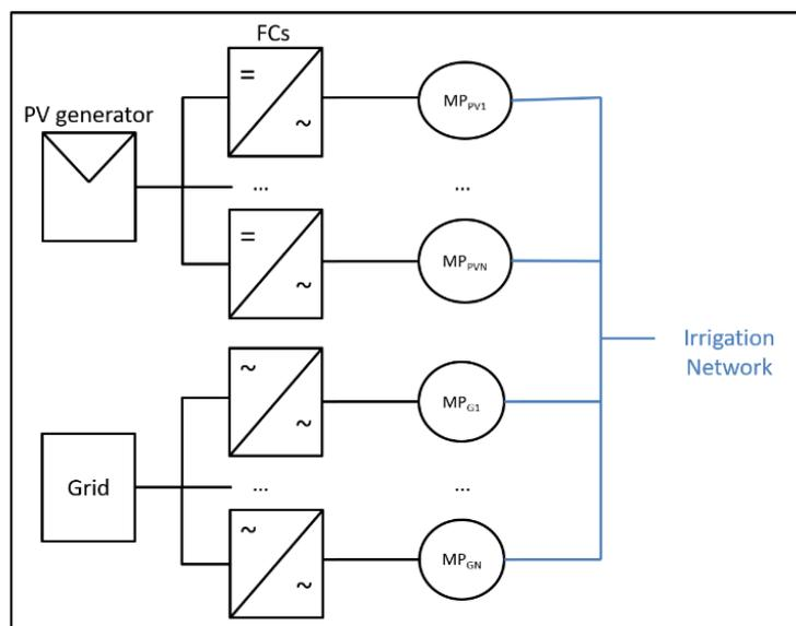
Figure 2 - Hydraulic hybrid systems: the irrigation system is fed by energy produced by PV generators but also from other sources (diesel or gas generator sets and conventional electricity grid), but hybridization is carried out into the hydraulic circuit.
