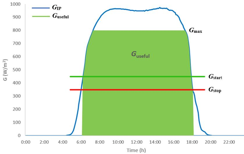
Figure 6. Graphical representation of the useful irradiance for a PV irrigation system working at a variable frequency.
