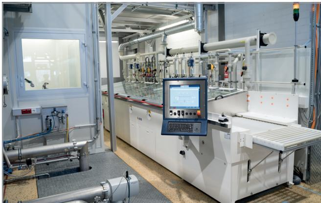
**Fig. 1: Ultrasonic wet cleaning line for ultra-thin glass**
