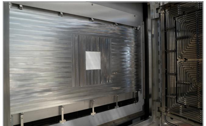
**Fig. 2: Example of an electrostatic chuck for fixing the ultra-thin glass during coating**
